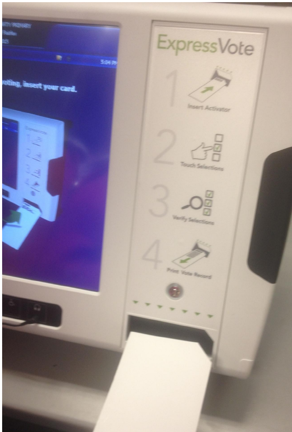
Ballot card for ExpressVote - notice that the corner cut of the ballot matches the insertion slot on the machine.
